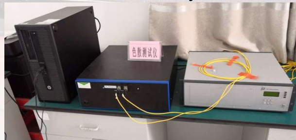
CD500 Chromatic Dispersion Measurement System
