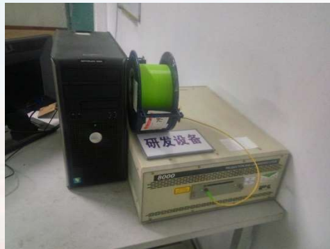
PK8000 Optical Time Domain Reflectometer (OTDR)
