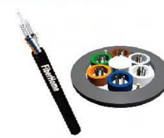
T-10 Loose tube stranded metal-free cable Outdoor Cable Stranded Cable-GYFTY
