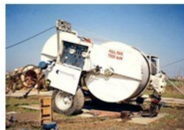
Picture 2: Active Hydraulic Tension Machine.
